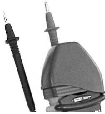
Fig. 3: Use of rubber test lead holster
