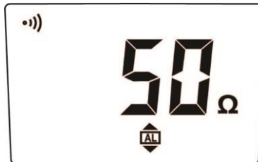
Fig. 33: Setting of alarm thresholds in resistance measurement
